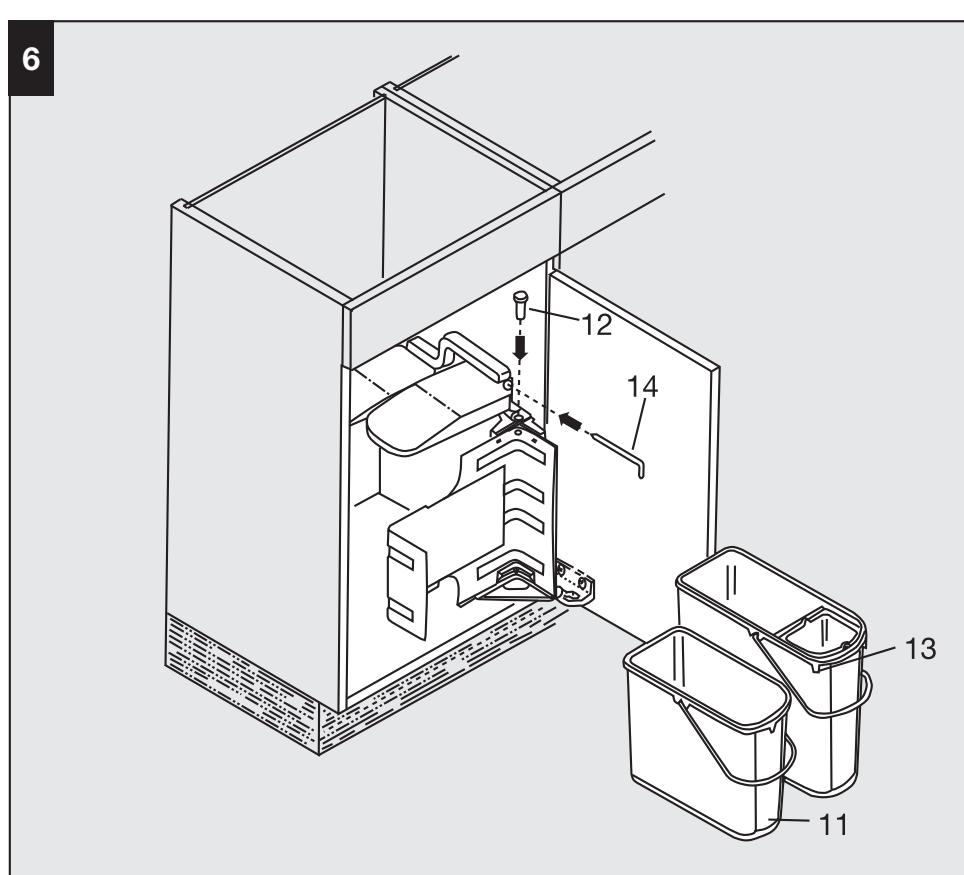
Fix cam (6) at the holding device for bin (7) with self-cutting screw 4 x 15. Press base shelf (8) on the holding device for bin (7) with a screw-driver; insert distance corner (9) and fasten with self-cutting screw 4 x 15. Fasten distance corner (10). Push in cam-follower (12).
