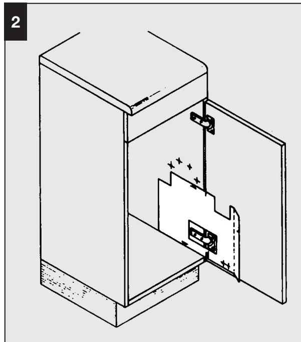
Line up template as shown in ill. 1 and 2 score fixing points for brackets and cam guide. Then pre-drill a 2 mm dia. drill bit.
